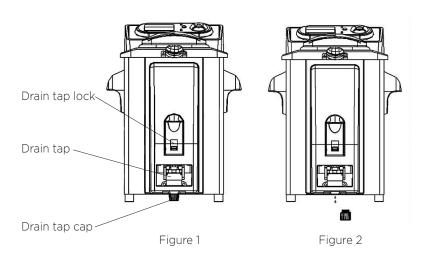
Your Wolfgang Puck Flash Fryer is equipped with a safety drain cap. Your drain tap cap should always be in place when using your deep fryer or when storing oil in the tank (see figure 1). The following directions outline the use of the drain tap.
